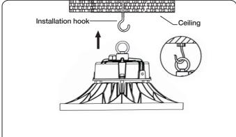
$\ensuremath{\mathsf{STEP}}\xspace$  3. Hang the circular rign onto the installation hook.
